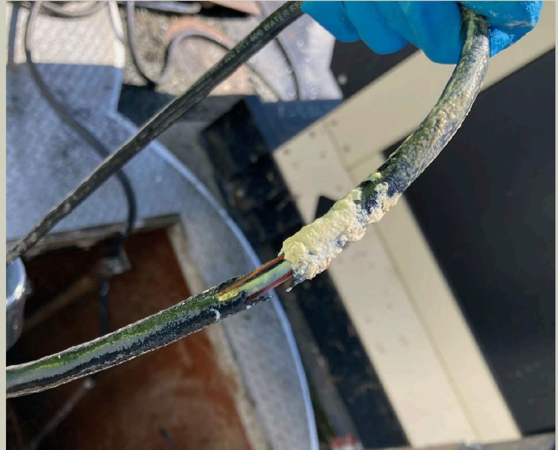
Replaced a failed float at LS 4 - Copper Cove
